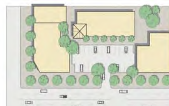
L32 Parking lot placement Unacceptable
