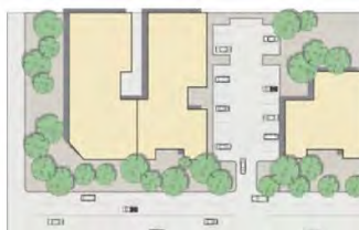
L31 Parking lot placement Acceptable
