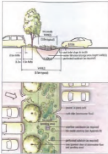
Design concept for bio-retention swale with tree planting
