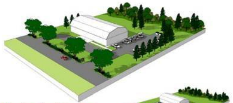
Best Practice: Combining the practice of orienting parking to the side or behind roadside development with the addition of screening along the roadway reduces the visual impact of parking and storage areas.
