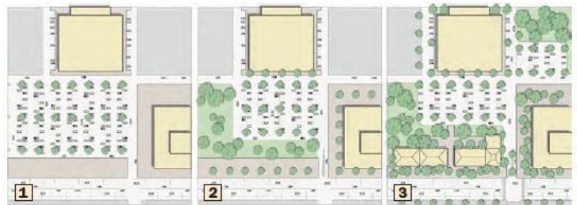
Image from The Community Design Manual, Ulster County Planning Board (March 2017) – shows the progressive redevelopment of an existing auto-oriented commercial corridor (1) with reduced parking, pedestrian improvements and enhanced landscaping (2); and eventually new sidewalk-oriented development along the roadway frontage (3).
