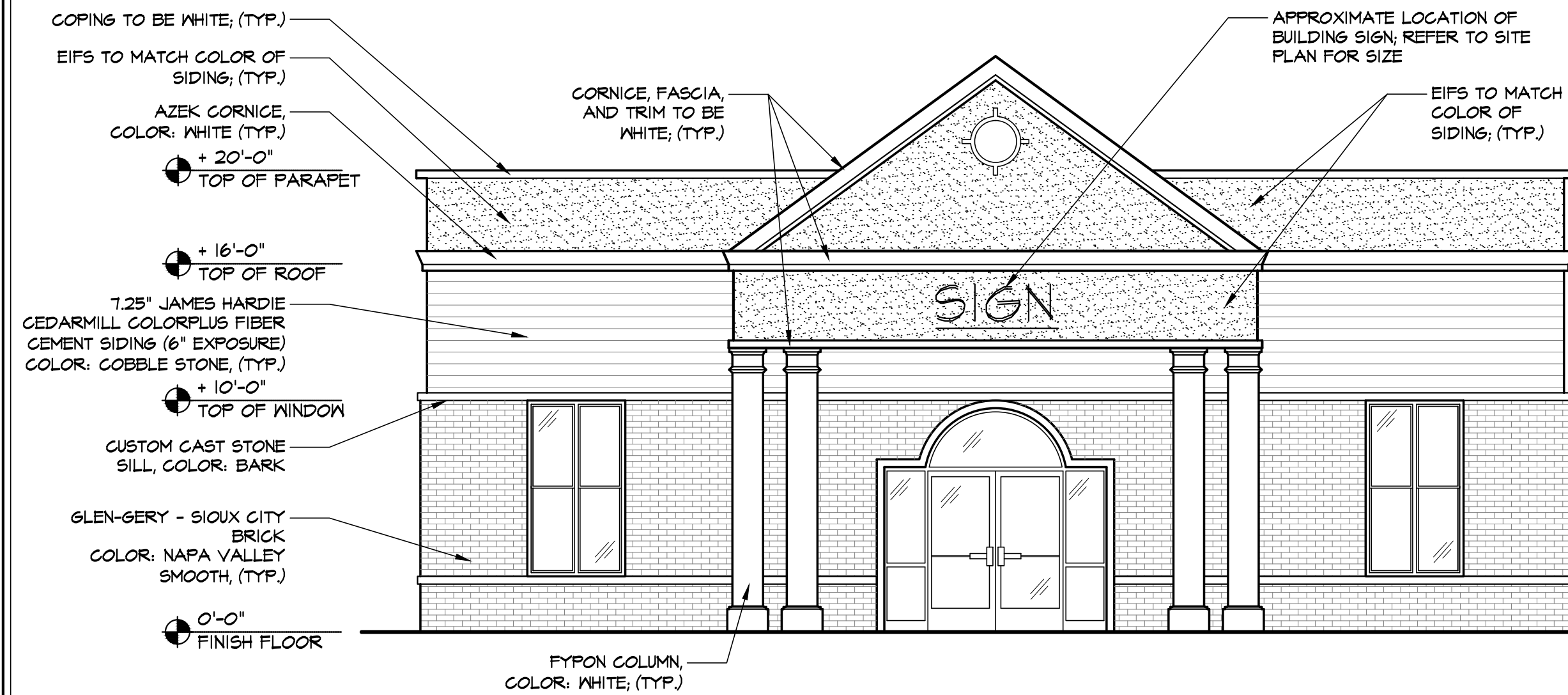
3 PROPOSED BUILDING #4 (BANK) - FRONT & REAR ELEVATION
