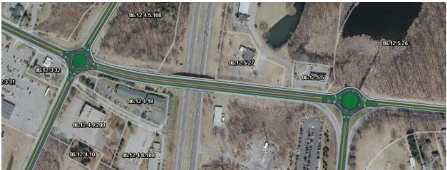
Creation of two roundabouts at the critical intersections could provide benefits to motorists, cyclists and pedestrians; improving safety for all, eliminating the need for a left turn lane on the bridge and allowing space on the bridge for a shared-use path.
